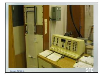
A key switch-initiates start up of SLOWPOKE to a preset power level, causes a single control rod to withdraw, system excess reactivity rises to 0.4% within < 8 seconds.
